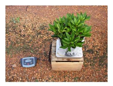
**Equipment needed for LF, ET and CF testing**: portable bench scale with range of 0-30 kg and a precision of at least 0.01 kg handles most situations. Approx. cost: \$500.
