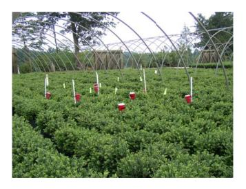
Fig. 2. Irrigation cups are placed above the canopy in the vicinity of test plants to determine irrigation rate applied during CF testing.
